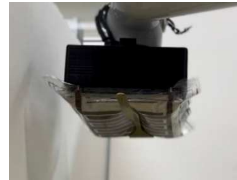
Multi-Gripper Technology Combining Jamming Gripper and Electrostatic Adhesion Technology
